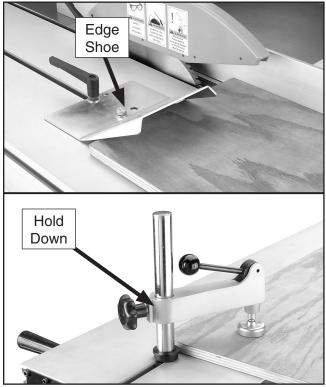
Figure 52. Edge shoe and hold down placement.
